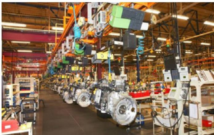
All fifty carriers have a Moby data tag attached. This stores an engine's build attributes and determines its route through the system.
